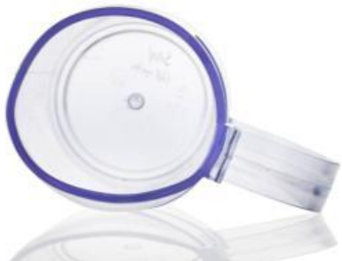
SAN after 125 cycles and no drop test
