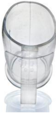
Methacrylate styrene after 50 dishwasher cycles and drop test
