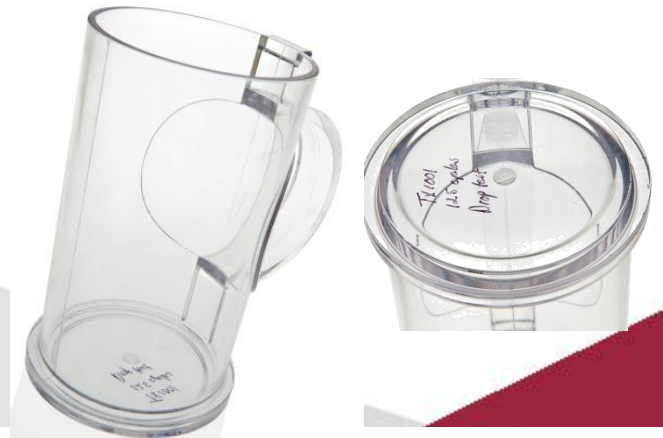
Eastman Tritan™ copolyester after 125 cycles and drop test: No effect
