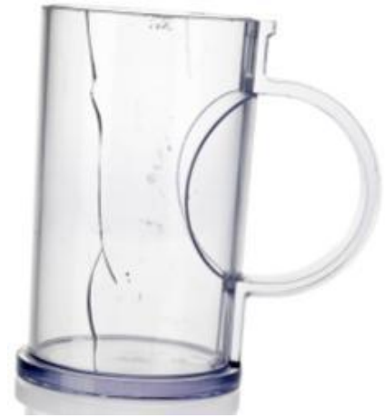
SAN after 30 cycles and drop test
