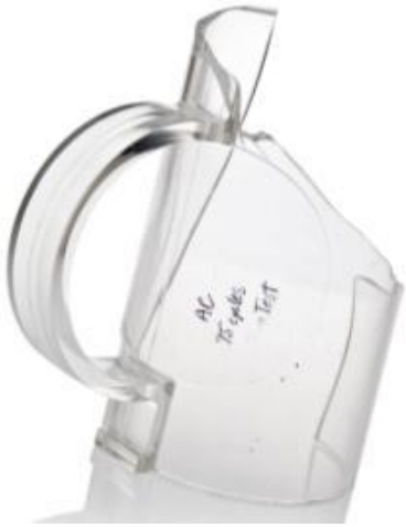
Acrylic after 75 dishwasher cycles and drop test
